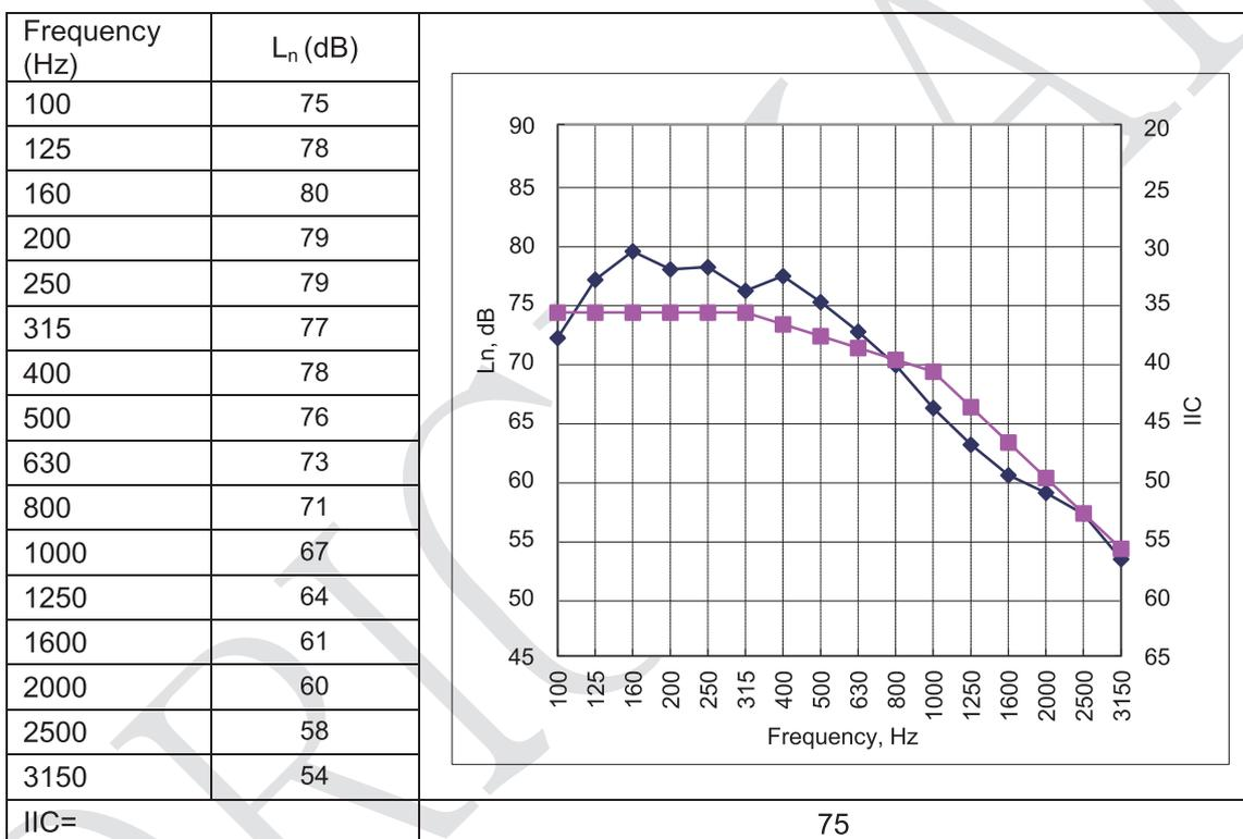
**Calculated Impact Insulation Class: IIC75**
